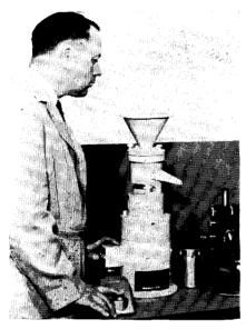
Throughput rates vary from 1 to 3 gal. per hour, depending on the material. Power is supplied by a 0.75 hp. motor.
